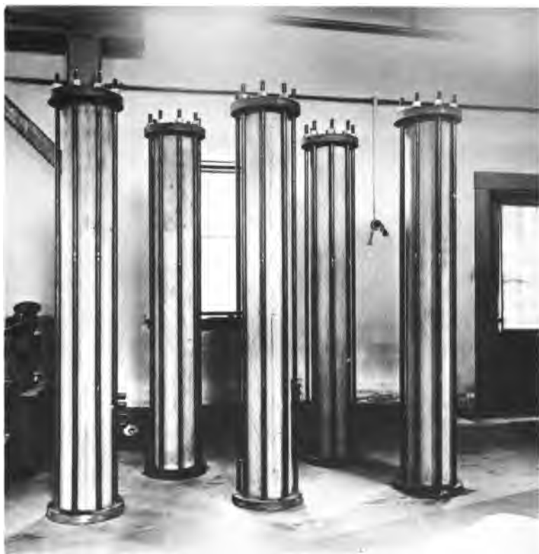
CONCRETE COLUMNS, PLAIN AND REINFORCED, SHOWING ARRANGEMENT OF SIDE-RODS AND END PLATES FOR SUBJECTING COLUMNS TO LONG CONTINUED LOADS.
